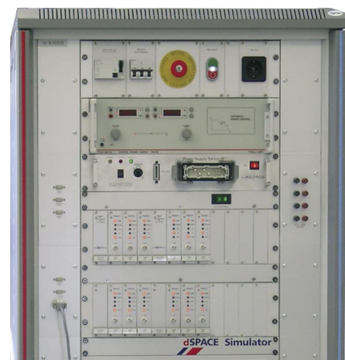
▲ Audi makes quick work of combining and recombining 152 infotainment components to test fault diagnostics. The developers switch component configurations on the dSPACE Simulator in next to no time, simulate fault cases, and perform restbus simulation of LIN/CAN ECUs.
